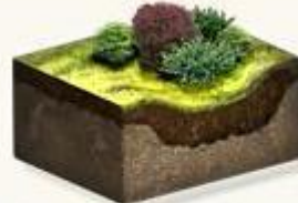
Rain Garden - Without Underdrain
