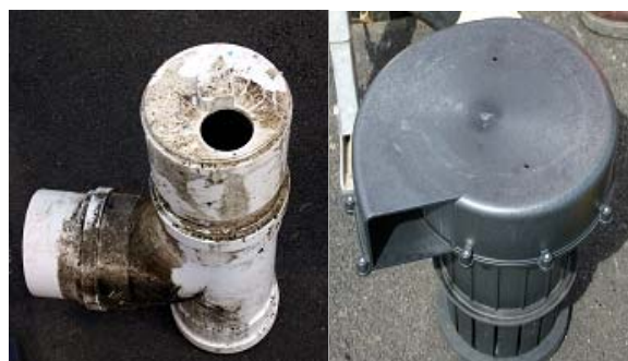
Hanging Trap (left, upside down showing orifice) and Vortex Unit (right)
