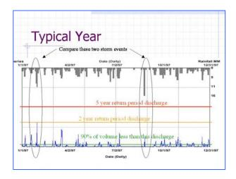
This hydrograph for a 'typical year' illustrate the variable response of a watershed to rainfall. Two events are highlighted in the graphic. The larger of the two rainfall events resulted in much less runoff. As can be seen from the hydrograph, the smaller of the two rainfall events was preceded by a period of wet weather such that more runoff resulted.
