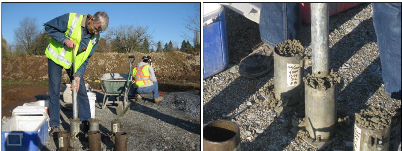
Fig. 5.1 – Cylinders were cast for measurement of unit weight, compressive strength and void content.
