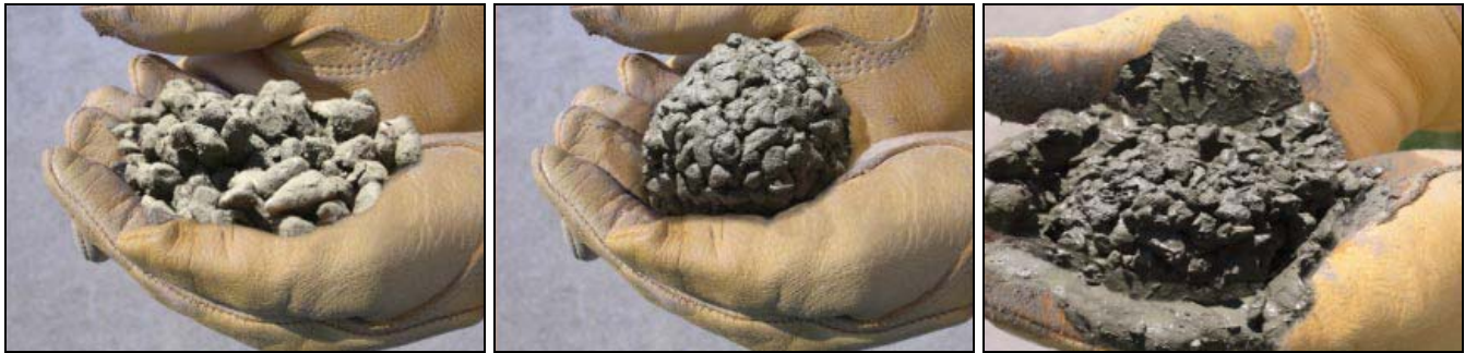
Fig. 2.1 - Samples of pervious concrete with different water contents, formed into a ball: (a) too little water, (b) proper amount of water, and (c) too much water.
