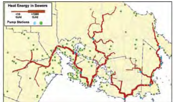
Figure 2 – Wastewater Heat Map for the Capital Regional District. Includes trunk sewers greater than 450 mm diameter.
